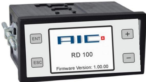
Display, calculate and log easily your instantaneous fuel consumption data, cumulative measured values as well as mass and CO2 emissions with 400 model. Remote display with a top intuitive handling.
